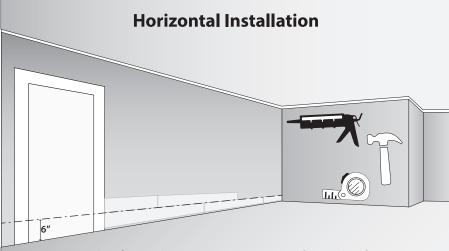
Starting on the floor, draw a level line at 6" from the floor. Next, attach the first plank in the left corner and add construction adhesive to the back of the plank then nail in place (see instructions above). Repeat this process until you reach the right wall cutting the pieces as needed. Stagger the next row of planks over the joints and cut pieces to fit as needed until you reach the ceiling. Finally add wood trim at the floor to finish your installation if desired.
