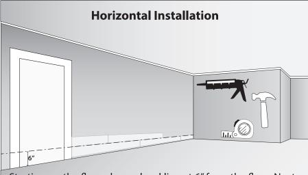
Starting on the floor, draw a level line at 6" from the floor. Next, attach the first plank in the left corner and add construction adhesive to the back of the plank then nail in place (see instructions above). Repeat this process until you reach the right wall cutting the pieces as needed. Stagger the next row of planks over the joints and cut pieces to fit as needed until you reach the ceiling. Finally add wood trim at the floor to finish your installation if desired.
