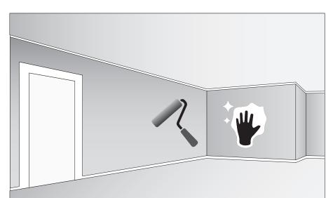
**Step 2)** Before installation, make sure that the surface is clean, flat, and dry. If you are installing over a sheetrock wall that is painted a color, we recommend that you paint the wall a similar color as the planking to be installed so the light color will not show through any possible seams between the planks.
