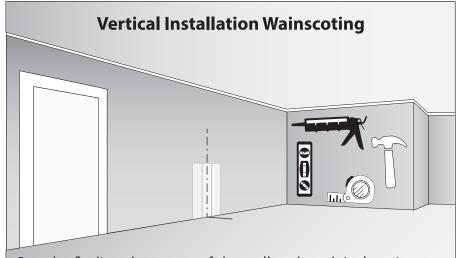
Start by finding the center of the wall and mark its location on the floor. Install the first plank on the wall centered on the mark with construction adhesive and nail in place with a brad gun (see instructions above). Use a level to make sure it is plumb. Next, attach planks on the left and right of first centered plank until you reach the corners of both walls. The width of the final plank at each corner will need to be trimmed to fit.
