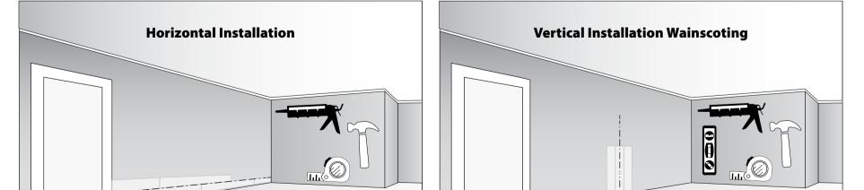
Starting on the floor, draw a level line 6" from the floor. Next, attach the first plank in the left corner and add construction adhesive to the back of the plank then nail in place (see instructions above). Repeat this process until you reach the right wall, cutting pieces as needed. Stagger the next row of planks over the joints and cut pieces to fit as needed until you reach the ceiling. Finally, add wood trim at the floor to finish your installation if desired.
